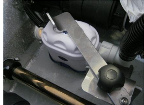
Automatic pump with locking arm
