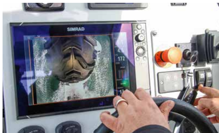
Bow and stern camera vision is relayed to the Simrad NSS12 screen monitoring wheel deployment.
