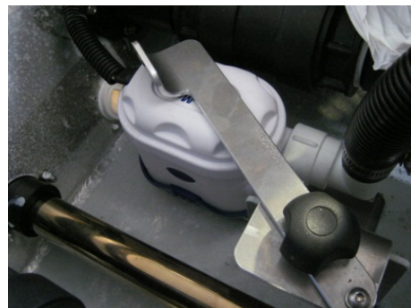
Automatic pump with locking arm
