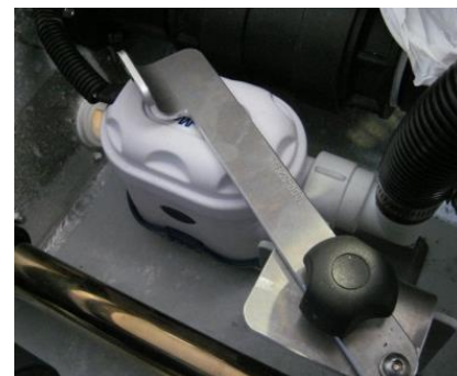
Bilge pump, with locking arm
