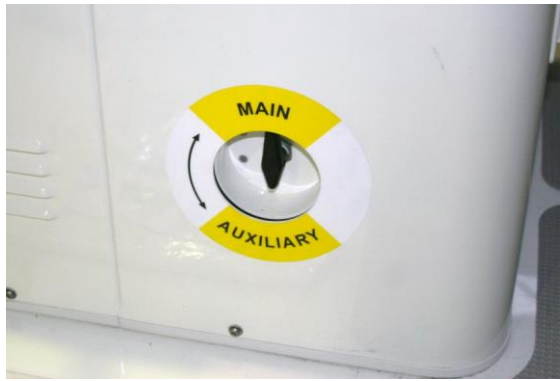
Main/Aux Tank Selector on Engine Box Cover
