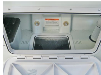
Transom locker and bilge access hatch
