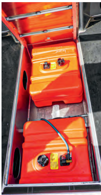
Left: Twin 45 litre tote tanks will fit underfloor. Above: To transport the Sealegs further afield, a Hosking trailer that fits the boat is available.
