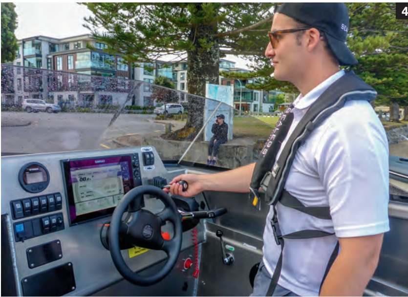
4) A rocker switch system will raise and lower the wheels, a gear-and-throttle lever controls the forward and reverse driving, a second throttle controls the engine revs and there is an emergency brake button too. 5) The well layed-out dash includes a Simrad MFD. 6) The transom locker also gives access to the bilge pump. 7) The new bait station made for the 6.1m by Manta Marine. 8) As a day fisher, the forecabin has no space wasted with berths. 9 & 10) The 130hp Yamaha Four Stroke outboard can push the boat to over 30 knots.
