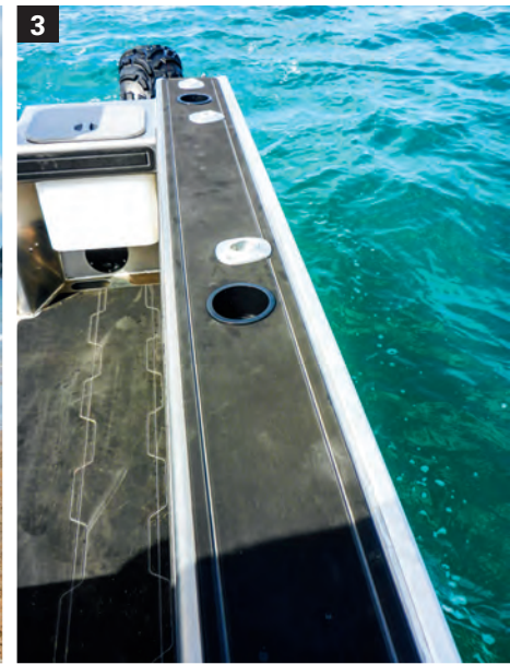
1) A mackerel-sized livebait tank is set into the transom. 2) A big advantage is quick, easy solo launching anywhere you can get beach access. 3) U-Dek covers the foredeck, gunwales and cockpit floor, providing good footing and a tidy finish.
