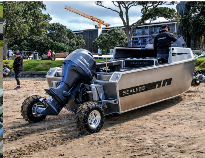
On shore, the wheels can be retracted for easier boarding and unloading.
