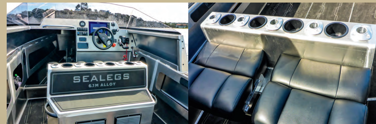
The central engine box doubles as seating with two single forward-facing fold-down bolster seats.
